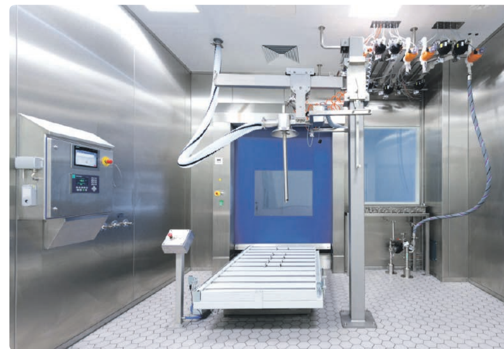
Clean room class GMP D for filling of liquid pharmaceutical precursors.
