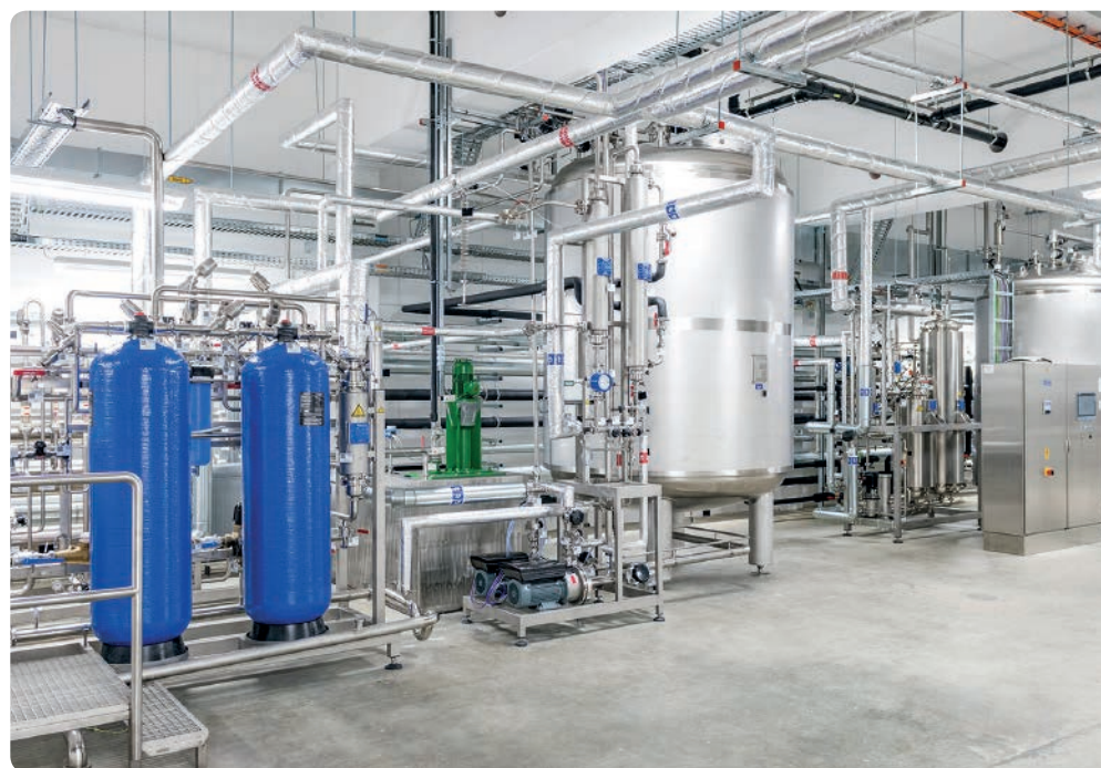
Production facilities for purified water and water for injection.
